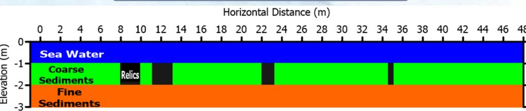
Figure 1: 2D section of the model used to create the synthetic seismic data.
