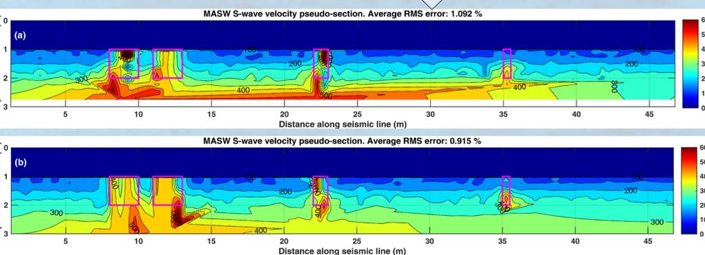
Figure 3: MASW S-wave velocity pseudo-sections deduced from synthetic data with (a) forward and (b) reverse source layouts, where forward and reverse source layouts refer to the position of the source, located in front of the first and behind the last receiver, respectively. The magenta rectangles delineate the positions of the relics. The color scale represents the Shear wave velocity (Vs).
