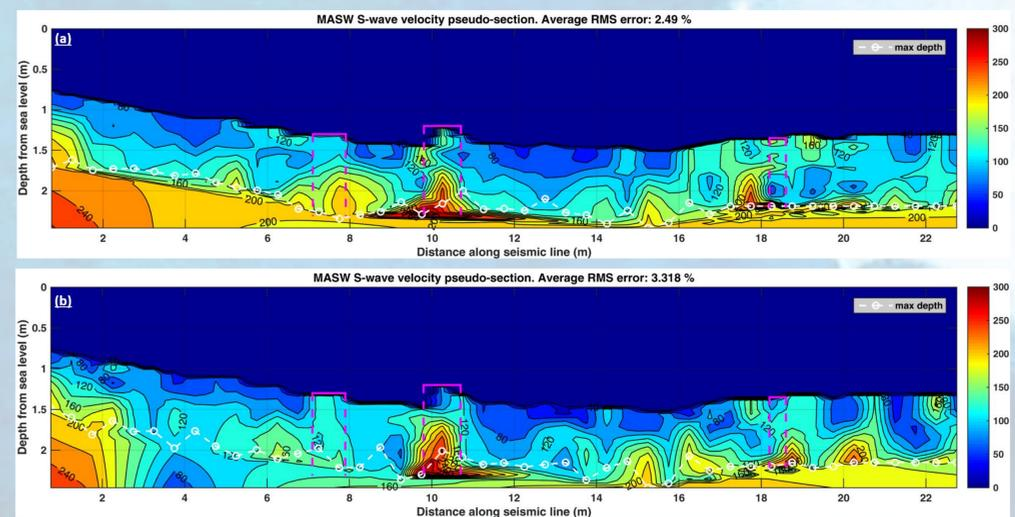
Figure 6: MASW S-wave velocity pseudo-sections deduced from the real data of Line 1 with (a) forward and (b) reverse source layouts. The magenta frames delineate the positions of the relics while the dotted white line with circles the max depth of investigation. The color scale represents the Shear wave velocity (Vs).
