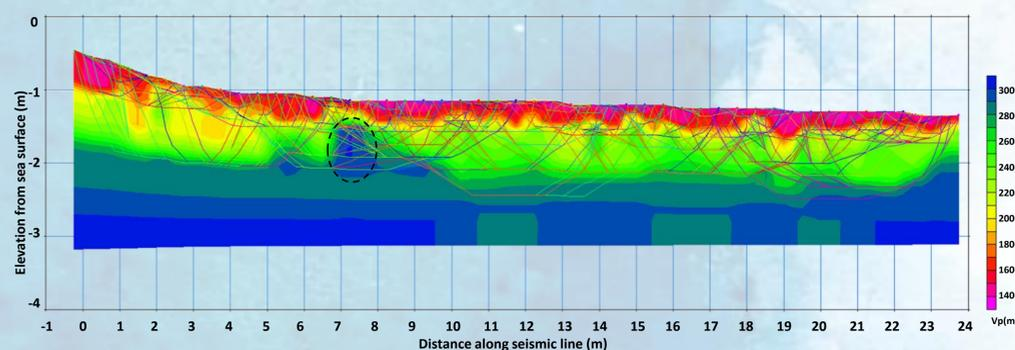
Figure 5: SRT P-wave velocity tomogram from the data of Line3. Dashed ellipse indicate a high velocity area, possibly attributed to buried submerged relics.
